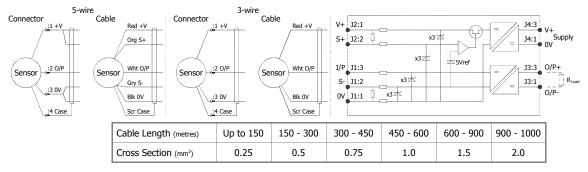
The table above shows recommended conductor sizes with respect to cable length for both three and five wire connections, based on copper conductors. Three wire connections will introduce a gain reduction of 5% and a  $\pm 1\%$  temperature dependence of gain over the range -40°C to +80°C for the cable temperature. (i.e. about -150 ppm/°C for the maximum lengths shown and less pro rata for shorter lengths.)
