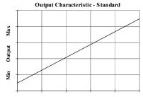
Retracted Linear Displacement Extended
